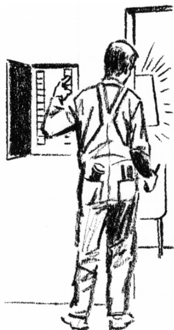
Figure 3.3 When you try to determine which electric circuit breaker supplies power to a particular light fixture, you turn on the switch of the fixture and then turn off the circuit breakers one at a time. In one of these "experiments" the bulb darkens, in the others it does not. Each turning off serves as a control experiment to be compared to the situation in which all circuits are turned on.
